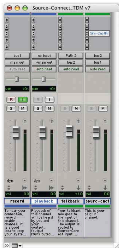
The template Session supplied by Source Elements illustrating how Source-Connect should be plumbed into a Pro Tools project.
